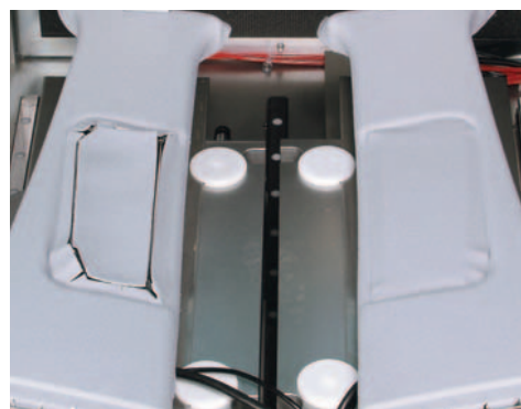
Twin unit for the simultaneous cutting and sealing of openings in automotive components.
