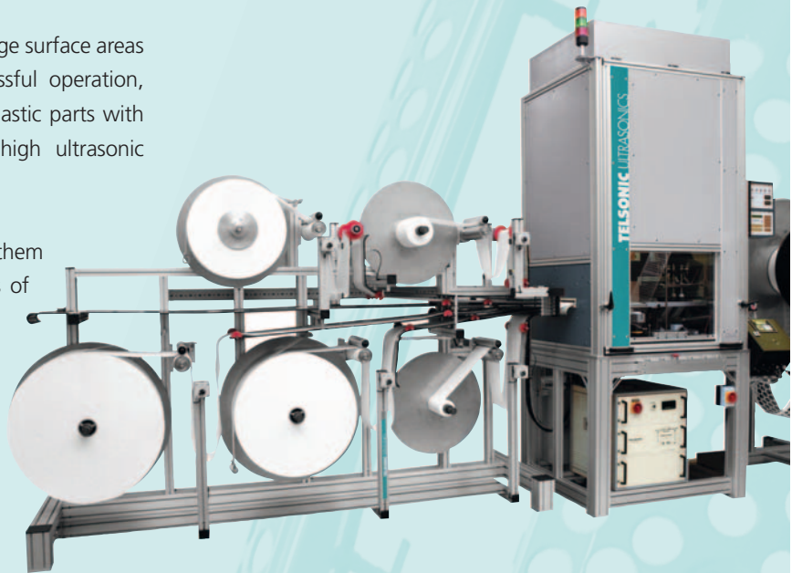
Fully automatic Cut'n'Seal machine for the manufacture of medical compresses in varying sizes and formats made up to 5 layers of material
