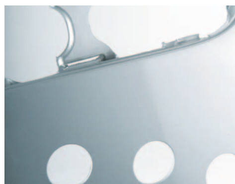
Automotive bumper with punched out openings for distance sensors
