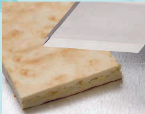
Cake with cutting sonotrode
